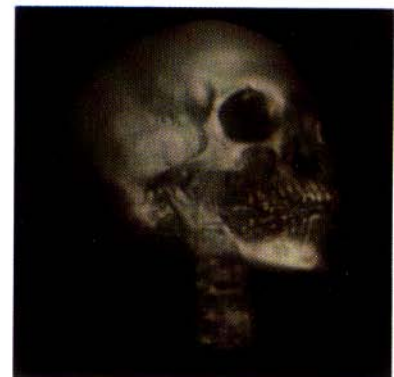
Figure 10: Volume rendering of the same data set as in Figure 9 using a ray-caster [12] for quality comparison (13.8 sec.).
