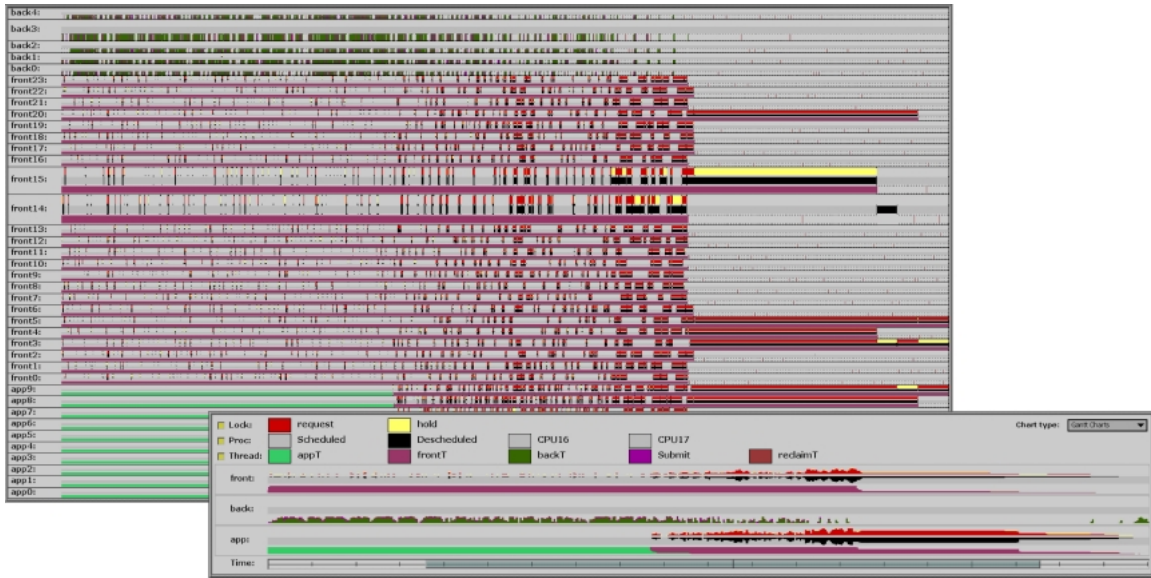
Figure 4. A visualization used in an iterative performance analysis of the Argus parallel rendering library. The visualization is shown displaying kernel lock, processor utilization and thread scheduling information for a 39-processor run of the Argus library. This data is shown in the top view using a stack of resizable and moveable Gantt charts. The bottom view shows these application events aggregated according to process type. The legend's color scheme can be directly manipulated; any changes are propagated to the charts via the listener mechanism. The checkboxes to the left of the legend control which event types are displayed in the top view. The time control in the bottom window acts as a dynamic query slider on the charts in the top window.
