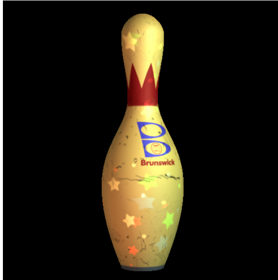
Figure 7: RenderMan bowling pin with 1 point light source and 4 animated textured lights. Since the shader is too large to map to a single pass, our RDS algorithm splits it into multiple passes. The pin renders at 30 frames/sec on a 1.4 GHz Pentium 4 system with an ATI Radeon 8500 graphics card.
