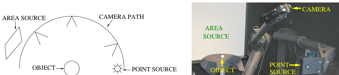
Figure 6.1: Left: Schematic of experimental setup Right: Photograph
