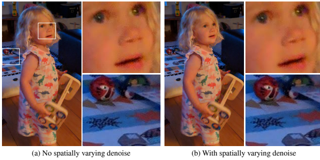
Fig. 10. Spatially varying denoising adaptively reduces more noise in regions with less temporal denoising, such as the face and hand. Static regions of the image are not affected. The amount of denoising increases in tiles with reduced frame merging.
