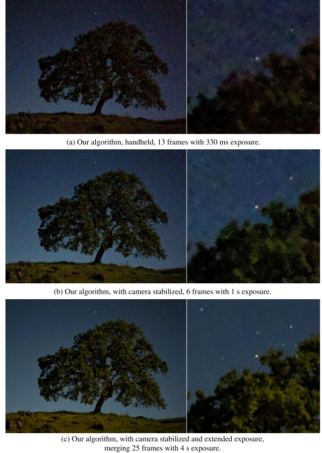
Fig. 5. A demonstration of our algorithm with extended exposures enabled by camera stability detection. The measured light levels at the tree were 0.06 lux. (a) A handheld capture uses 13 \times 333 ms exposures. (b) When stabilized on a tripod, our algorithm uses 6 \times 1 s exposures. The longer individual exposures greatly reduce noise. (c) Camera stability detection could be used for even longer captures, such as the 25 \times 4 s exposures in this example. Noise is significantly reduced, at the cost of a much longer total capture time.
