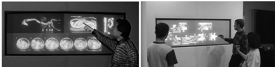
Fig. 1. A large visualization display on which multiple users can interact using laser pointers.
