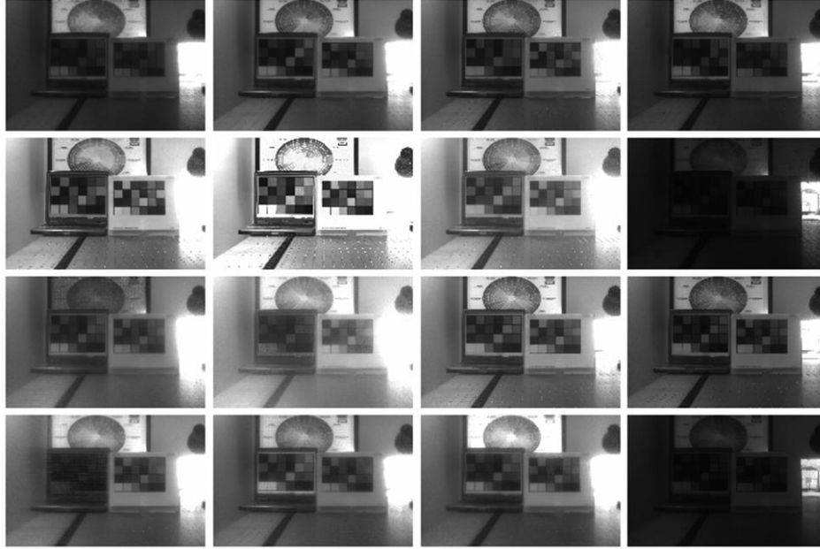
Figure 8: Sixteen images created from a single frame using the 16-filter configuration in Fig. 7(d). The resolution of each image is 177 x 117. The filters corresponding to each image are (from left to right): first row: blue, green, magenta and cyan; second row: red, no filter, yellow and infrared-pass; third row: 0° polarizer, right circular polarizer, 0.4 OD filter, 0.6 OD filter; fourth row: 45° polarizer, 135° polarizer, 90° polarizer, 1 OD filter. Images are arranged in the same configuration as the filters in the pupil plane.
