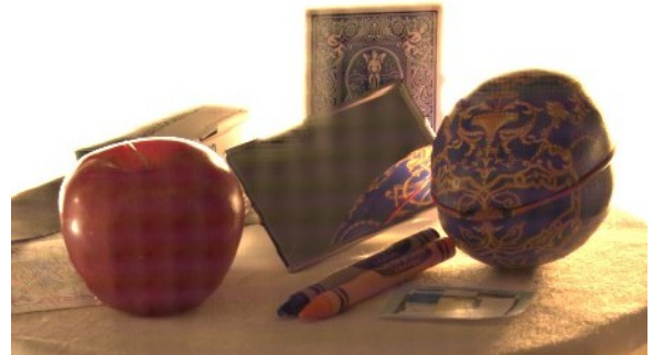
Figure 8: Periodic artifacts in direct/global separation. The pattern is aligned to the mask orientation and strongest near large brightness gradients, but is visible across most of the scene.
