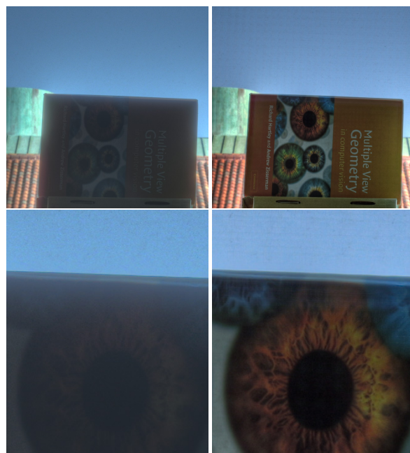
Figure 13: Tonemapped images of a book in a dark room, against a bright window showing a neighboring building and blue sky, captured with the Canon A640. At the top left is the unmasked HDR capture, and at the top right is our glare-free result. At the bottom is a closeup of corresponding regions from each capture. Compare to the deconvolution result in Figure 6.
