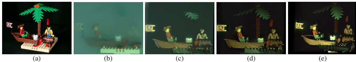
Figure 1: Reconstructed volume of a 3D scene in a fish tank with diluted milk. While in the floodlit image (b) only the front objects are recognizable, confocal imaging (c) partially removes the haze. Using our novel descattering algorithm combined with confocal imaging more global scattering is removed and objects at even larger distances become visible (d). The image is sharper and features more saturated colors. In (e), the recovered 3D structure is visualized for a different view. Images (c)-(e) have been created by computing a confocal or descattered confocal volume followed by maximum intensity projection.
