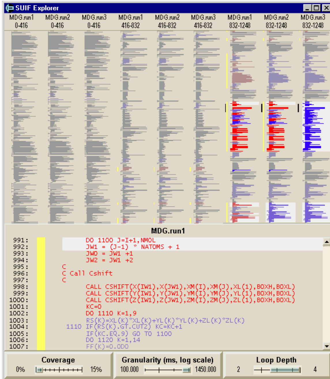
Figure 3.2: SUIF Explorer visualization showing three runs of the MDG molecular dynamics application, demonstrating how user intervention improved the parallel coverage of the application.
