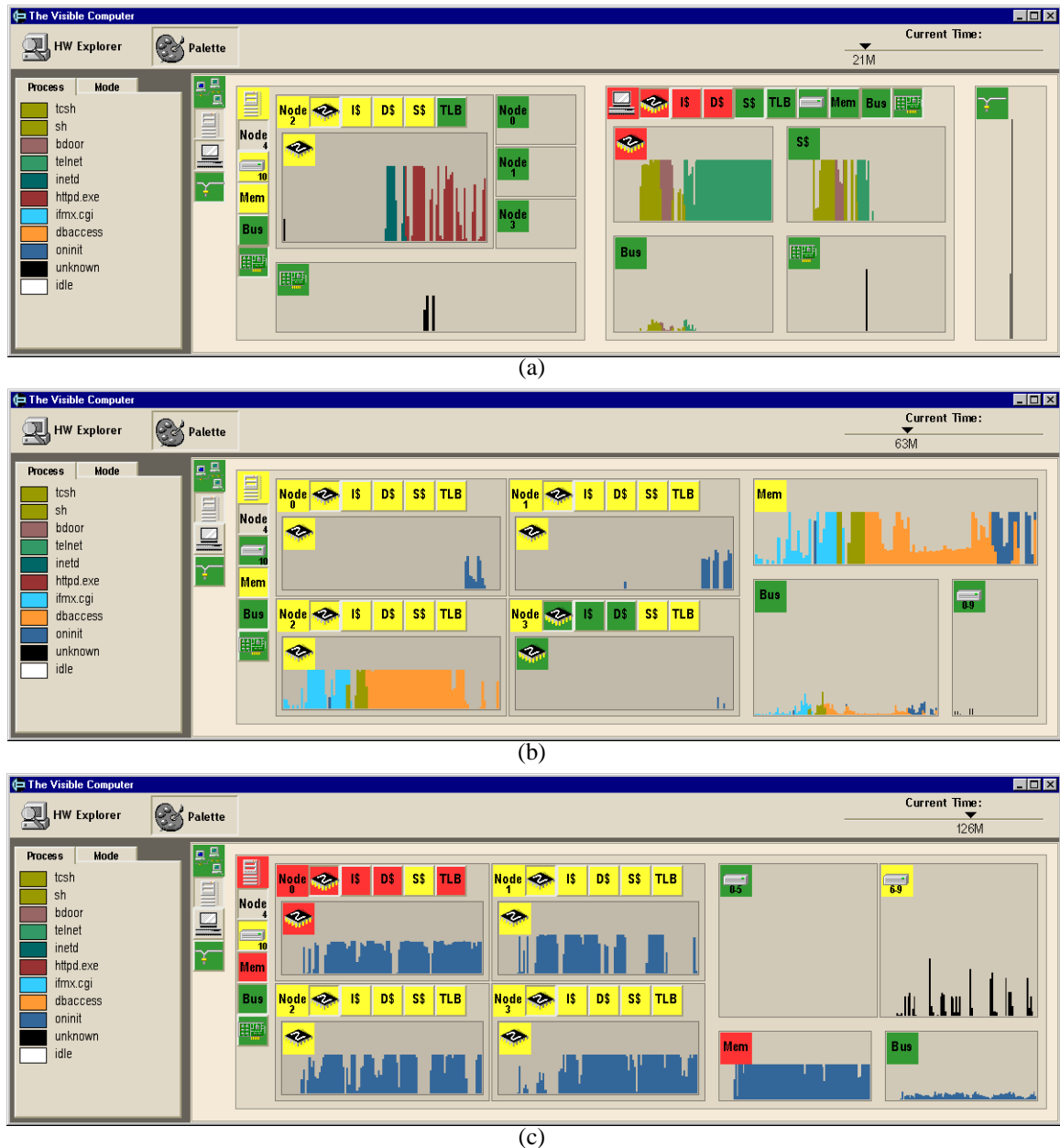
Figure 6.5: Sequence of screenshots from a Visible Computer analysis of a client-server database Web application. (a) Cycle 21M: Client issues database query to server via HTTP. Server node two begins processing the request, and the client incurs significant CPU busy time and cache stall time while waiting for response. (b) Cycle 63M: CGI script on server node two parses the Web query and launches the database access application dbaccess , which triggers the parallel database server process oninit on the other nodes. (c) Cycle 126M: oninit continues running on all four nodes. The server incurs significant memory stall time, and the disks containing the database (6–9) are frequently accessed.
