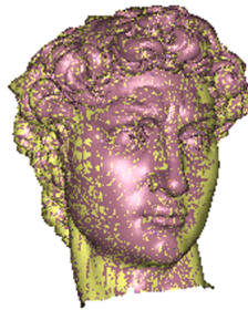
Figure 11: During view dependent rendering, the generated points are colored according to the level of their node.
