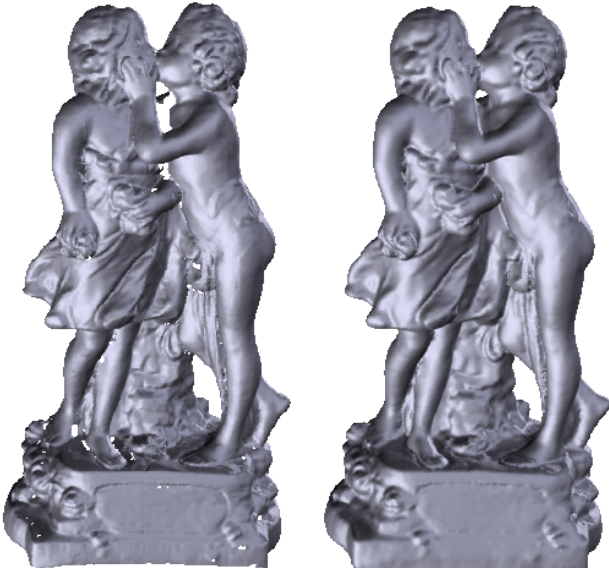
Figure 11: An RBF has automatically filled small holes and extrapolated across occluded regions in the scan data (left), to produce a closed, water-tight model (right). The complex topology of the statue has been preserved.
