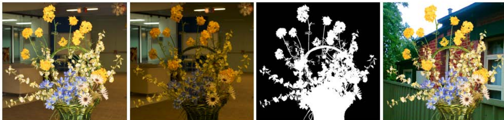
Figure 1: Flash matting results for flower scene with complex foreground and background color distributions. From left to right: flash image, no-flash image, recovered alpha matte, and flower basket with new background.
