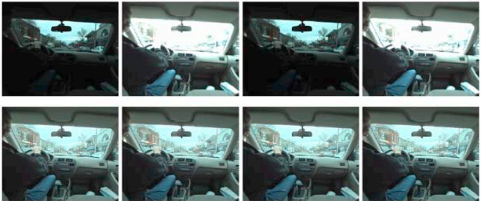
Figure 1: High dynamic range video of a driving scene. Top row: Input video with alternating short and long exposures. Bottom row: High dynamic range video (tonemapped).
